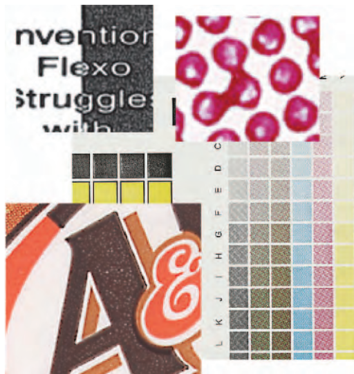
Flexo printing can have some poor quality results with conventional round dot screening.
